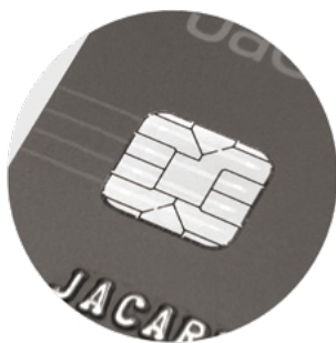
After 1,000 insertion cycles (any inexpensive s/c reader, typically with sliding contacts)
